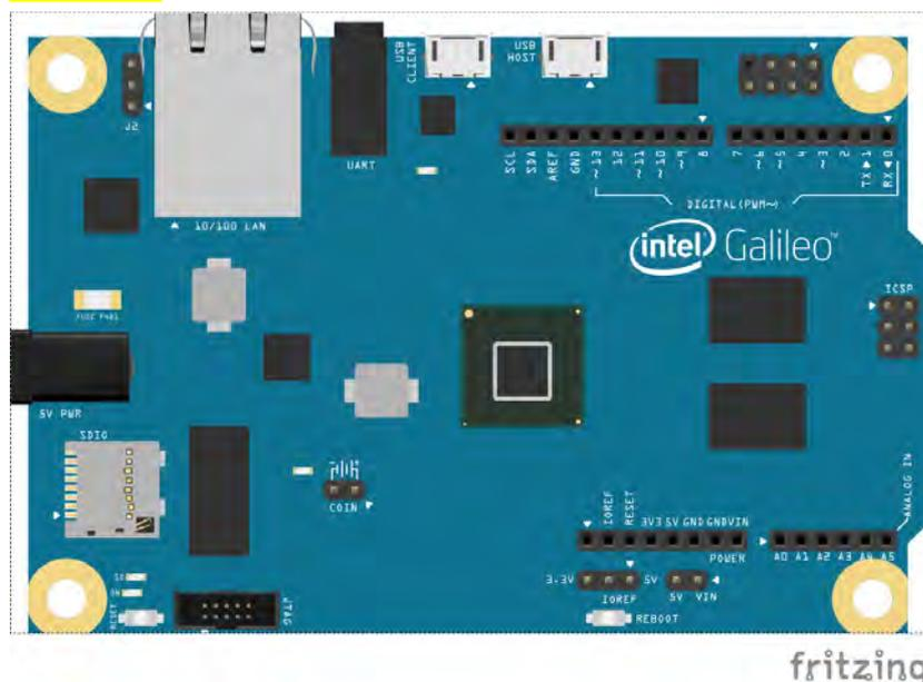
Fig 2.17 – Arduino Galileo.
