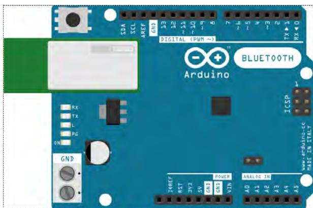
Fig 2.16 – Arduino BT.
