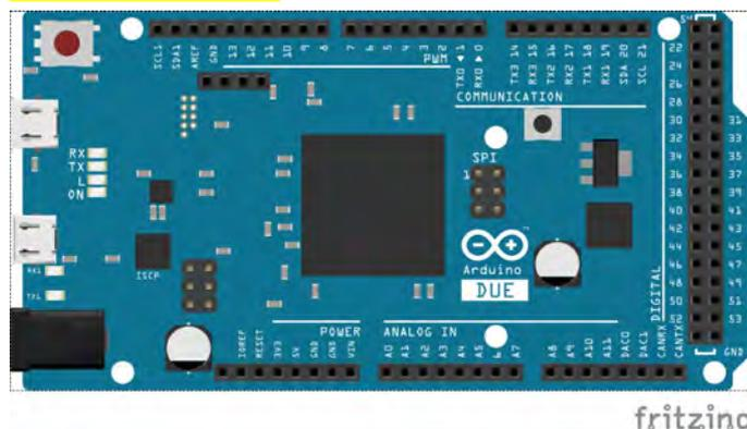
Fig 2.5 – Arduino DUE.
