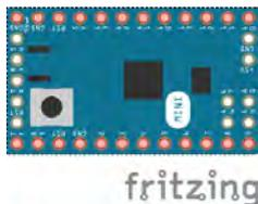
Fig 2.8 – Arduino Mini.
