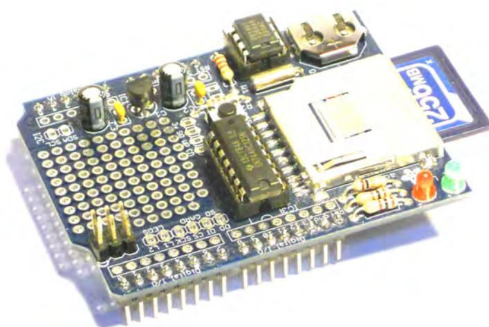
*Fig 2.18 – Data Logger Shield.*
