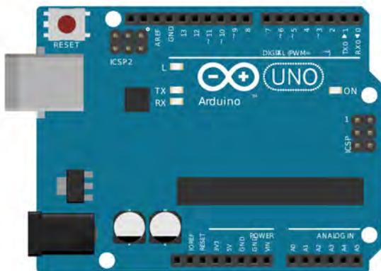
Fig 2.1 – La scheda Arduino UNO (Fritzing).
