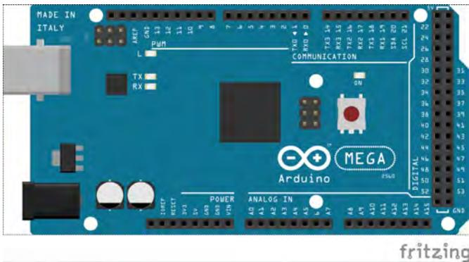
Fig 2.2 – Arduino Mega 2560.
