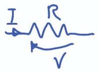
$$\begin{cases} P = V \cdot I \\ I = V/R \end{cases} \rightarrow P = \frac{V^2}{R} \rightarrow X = 10 \log \frac{P_a}{P_b} = 10 \log \frac{V_a^2/R}{V_b^2/R} = 10 \log \left( \frac{V_a}{V_b} \right)^2 = \boxed{20 \log \frac{V_a}{V_b}}$$
