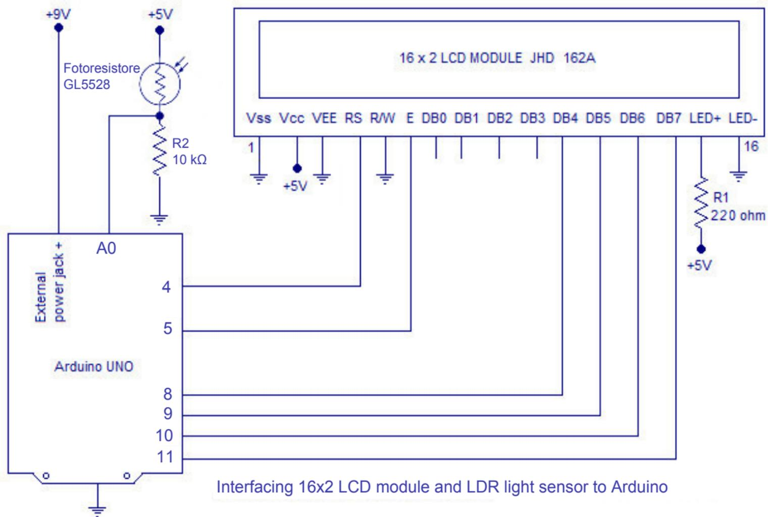
Interfacing 16x2 LCD module and LDR light sensor to Arduino
